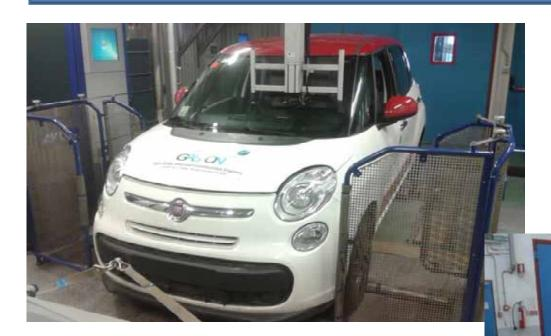
Measured driving (NEDC) range = 590 km Measured driving (WLTC) range = 550 km
