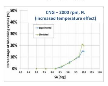
Knocking model prediction is confirmed by engine testing
